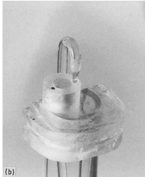
Figure 2 (a) Profile measurements are performed with a thermo-mechanical analyser (Mettler TMA 40). A close up of the quartz measuring probe is shown in (b). With the quartz measuring probe the surface of the calcium phosphate containing tube is probed on five points to measure the differences in height between the points.
