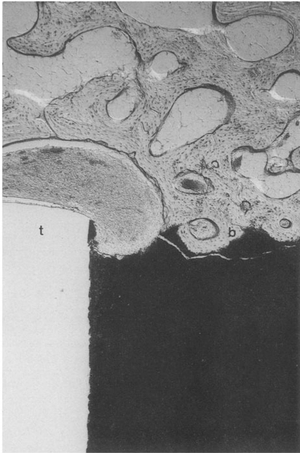
Figure 9 In contrast to Fig. 8, rhenanite (black) is shown after 3 months to have intimate contact with bone, while initial resorption has taken place. This implant cylinder was originally meant for profile measurements. No resorptive cells were found. (b, bone; t, acrylic tube; undecalcified section; \times 10 .)
